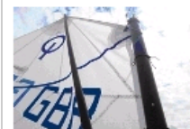
Fig.1 Head tie too loose
