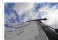
Fig.3 Luff too tight
