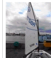
Fig.4 Outhaul not tightened
